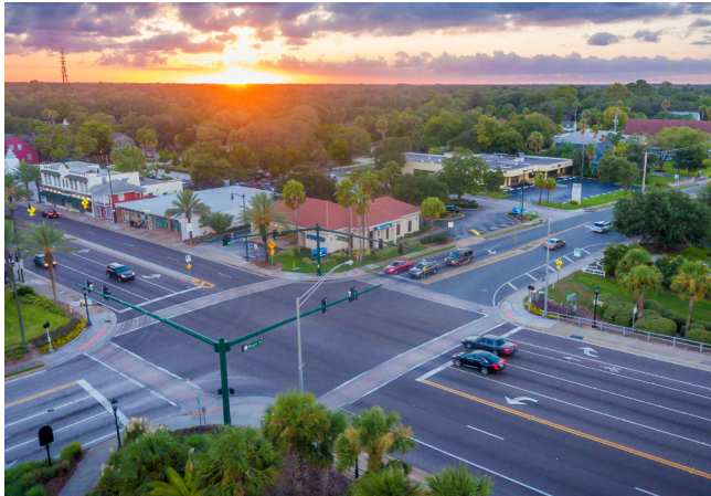
Figure 22. Dedicated Left- and Right-Turn Lanes at Intersections
