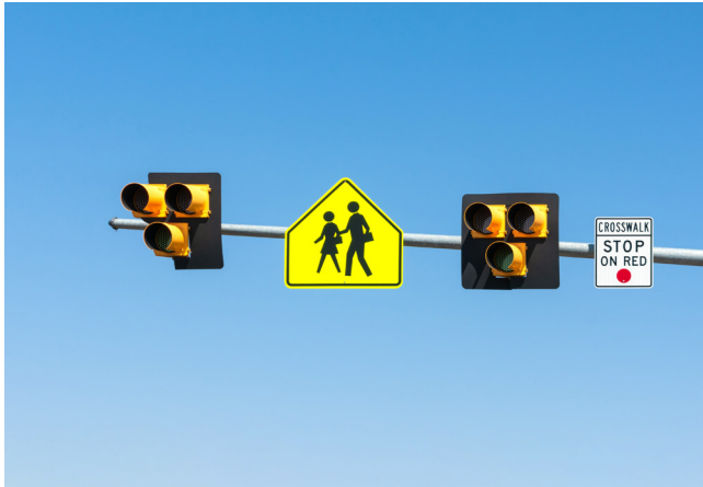
Figure 26. Pedestrian Hybrid Beacon
