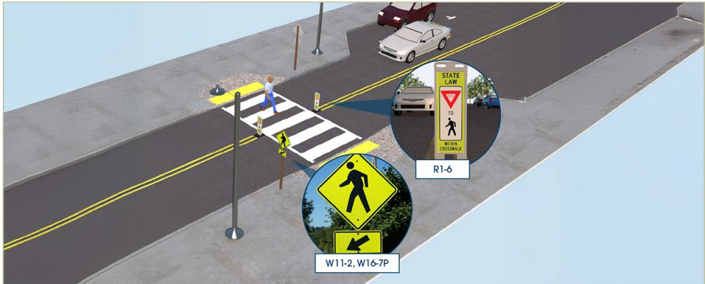
FIGURE 25. CROSSWALK VISIBILITY ENHANCEMENTS
