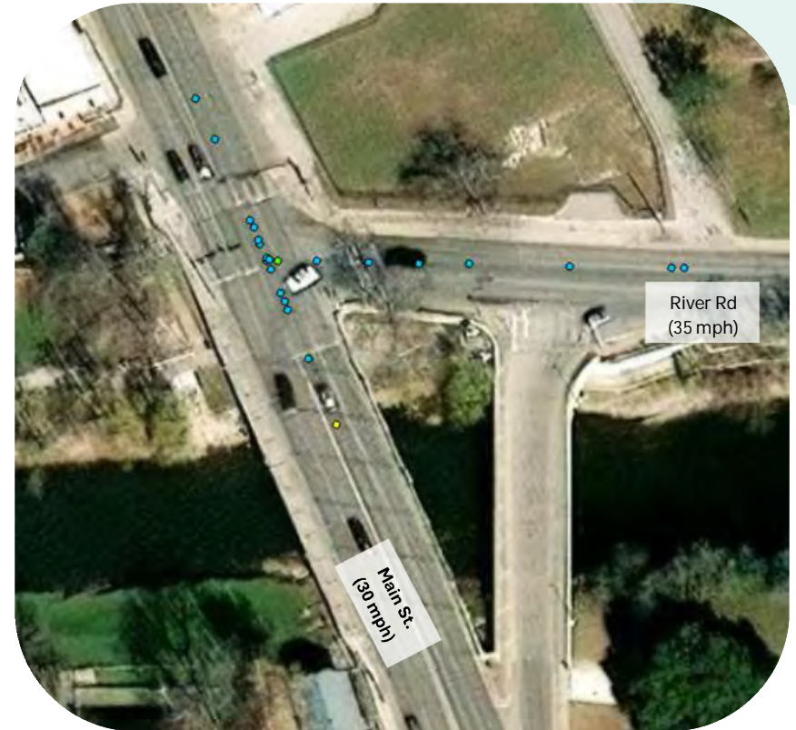
Crash history from TxDOT Crash Records Information System C.R.I.S. 2020-2024, based on crashes reported within 250 ft of intersection center.
